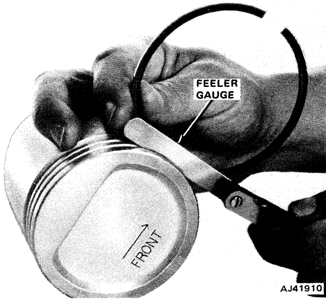
Fig. 1A-45 Ring Side Clearance
